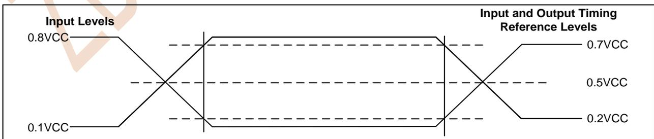
Figure 8.3 AC Measurement I/O Waveform
