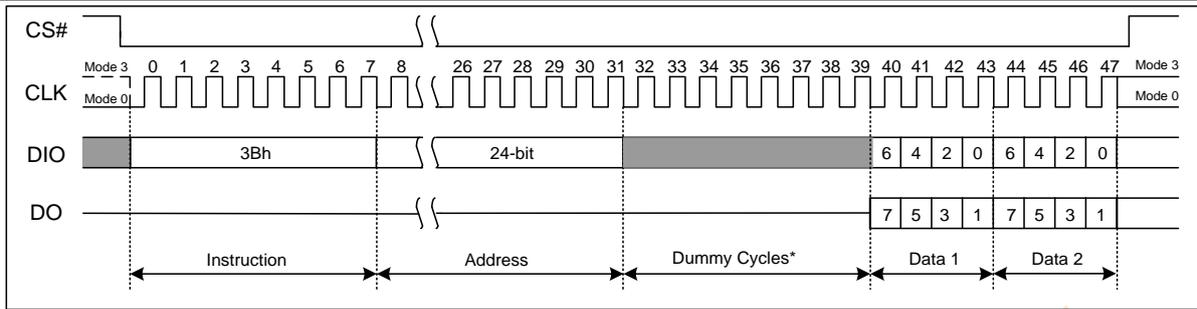
Figure 7.15 Fast Read Dual Output Instruction Sequence Diagram
