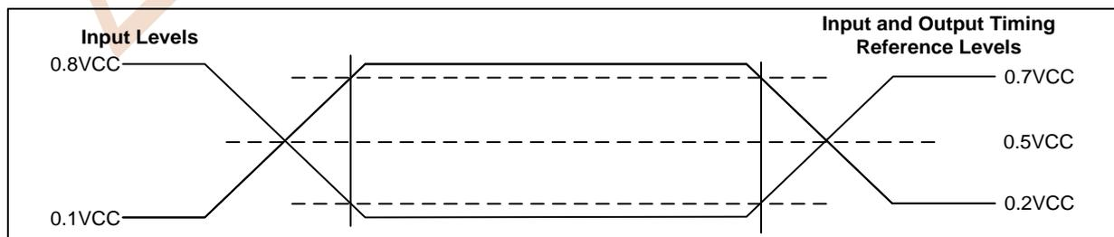
Figure 8.3 AC Measurement I/O Waveform
