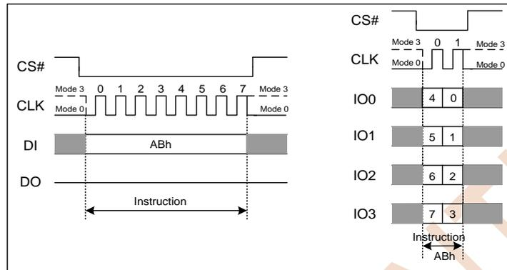
Figure 7.28 Release Power-down Instruction(SPI and QPI Mode)
