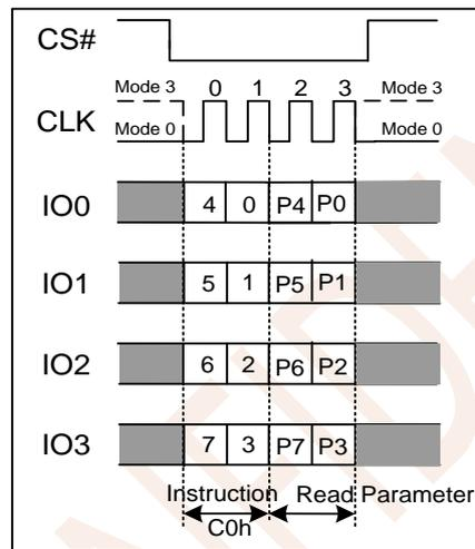
Figure 7.34 Set Read Parameters Instruction (QPI Mode only)
