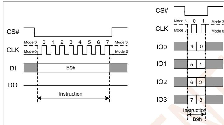
Figure 7.22 Deep Power-down Instruction(SPI and QPI Mode)
