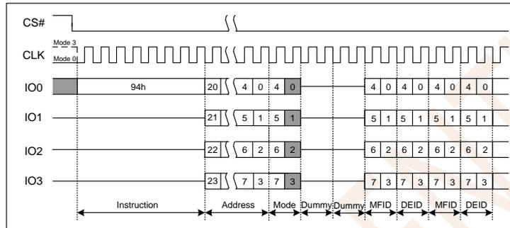
Figure 7.32 Read Manufacturer/Device ID Quad I/O Instruction
