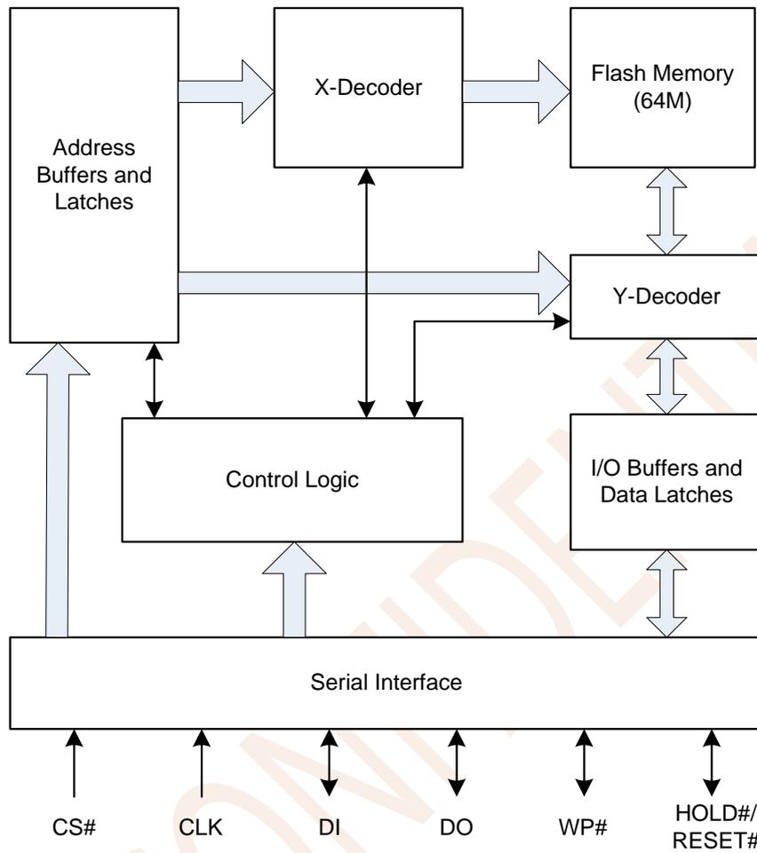
Figure 2.1 Block Diagram
