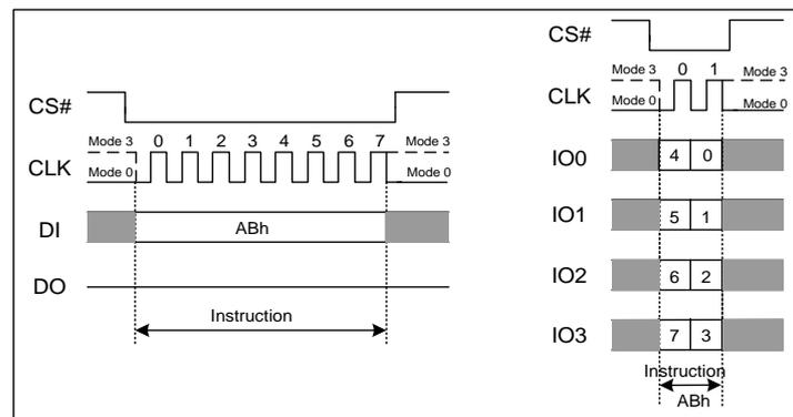
**Figure 7.23 Release Power-down Instruction(SPI and QPI Mode)**
