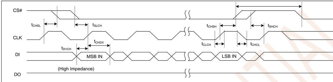
Figure 8.5 Input Timing
