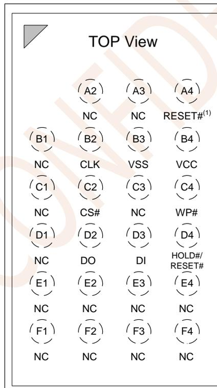
Figure 3.5 24-BALL TFBGA (6x4 ball array)
