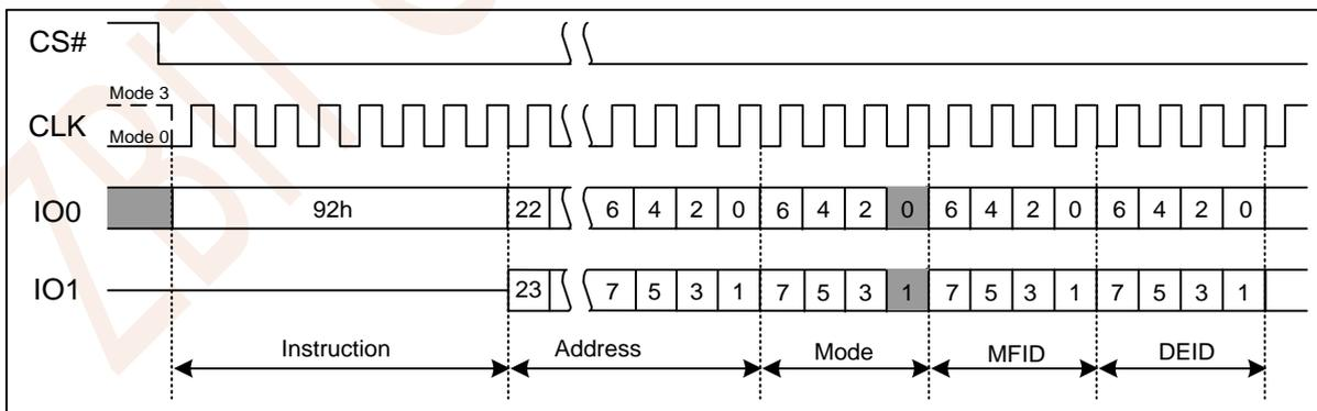
Figure 7.31 Read Manufacturer/Device ID Dual I/O Instruction
