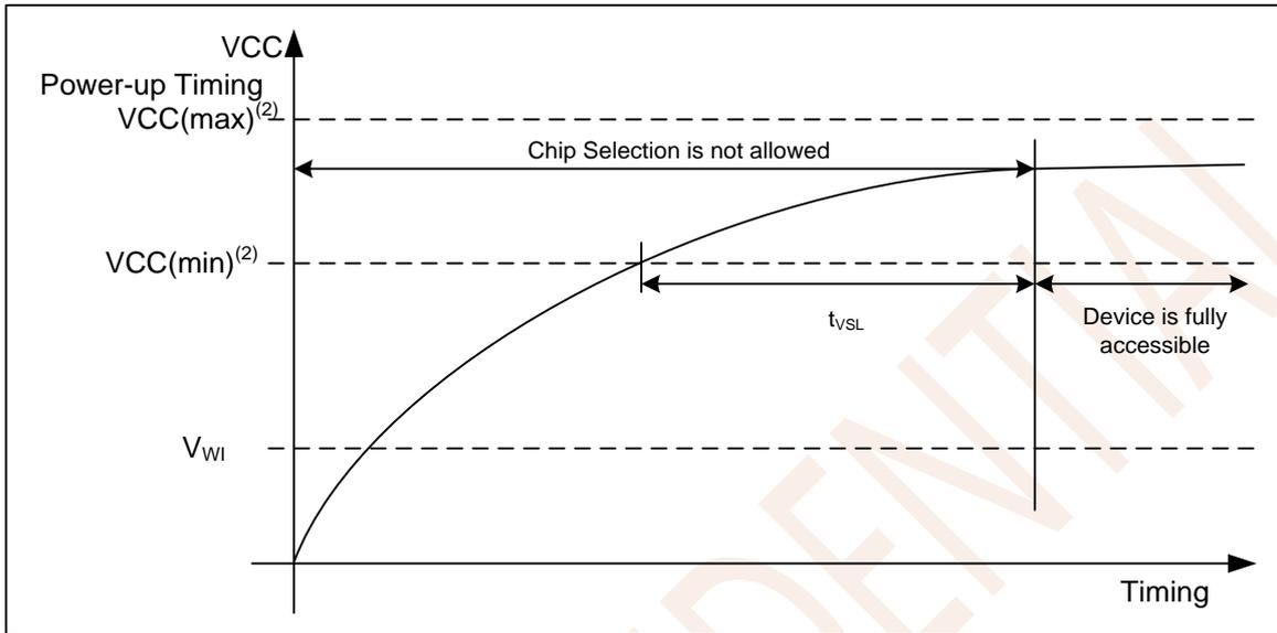
Figure 8.1 Power-up Timing
