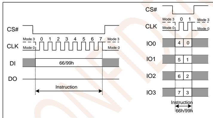
Figure 7.21 Software Reset Instruction(SPI and QPI Mode)
