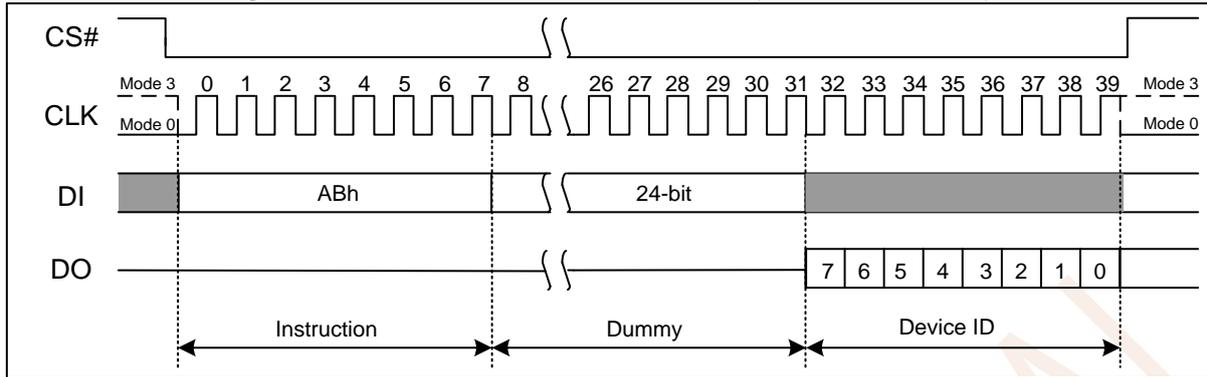
**Figure 7.24a Release Power-down / Device ID(SPI Mode)**
