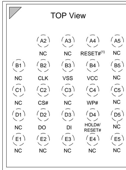
Figure 3.4 24-BALL TFBGA (5x5 ball array)
