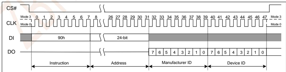
Figure 7.30a Read Manufacturer/Device ID(SPI Mode)
