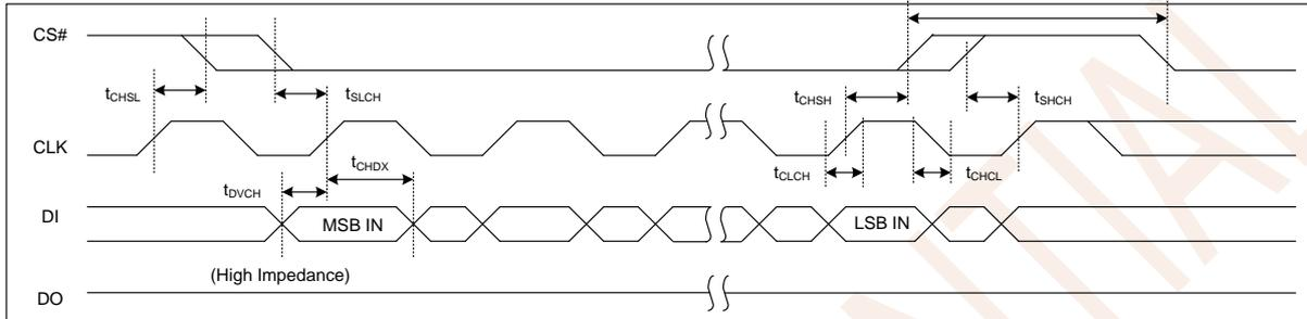
Figure 8.5 Input Timing
