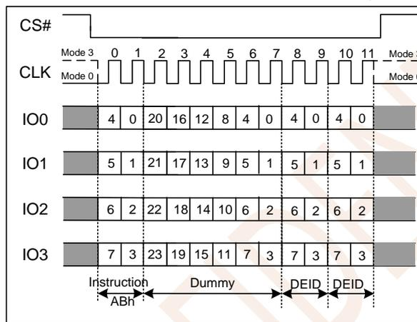
Figure 7.29b Release Power-down / Device ID(QPI Mode)
