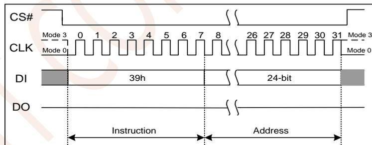
Figure 7.37a Individual Block/Sector Unlock Instruction(SPI Mode)
