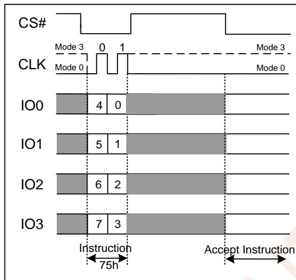
Figure 7.11b Erase / Program Suspend Instruction(QPI Mode)
