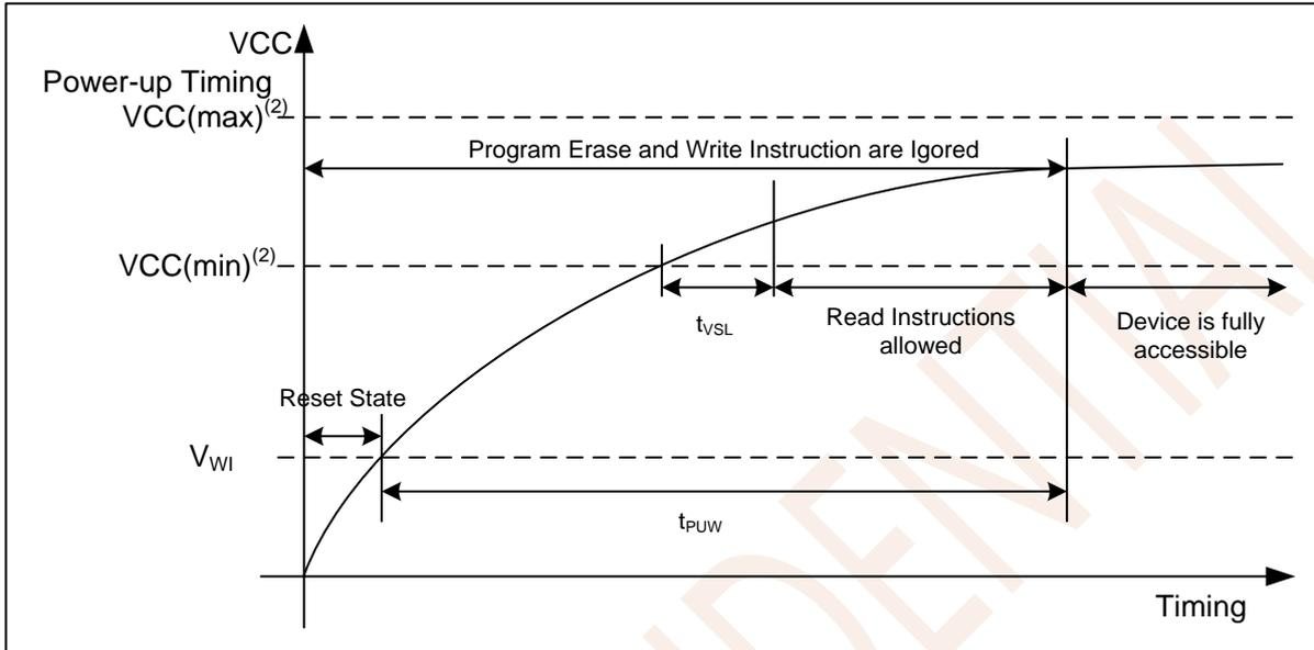
Figure 8.1 Power-up Timing
