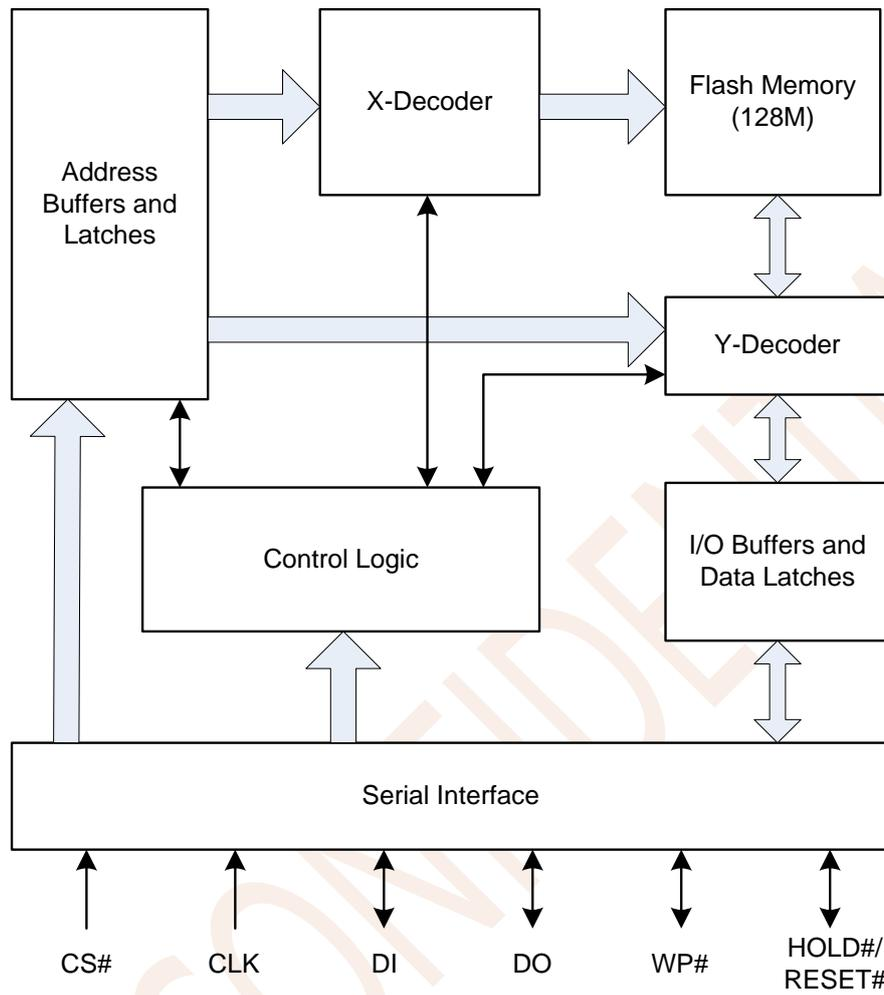
Figure 2.1 Block Diagram
