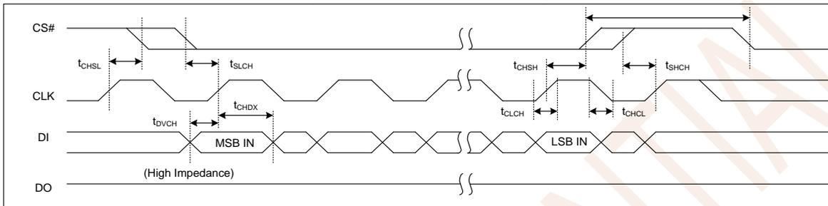
Figure 8.5 Input Timing
