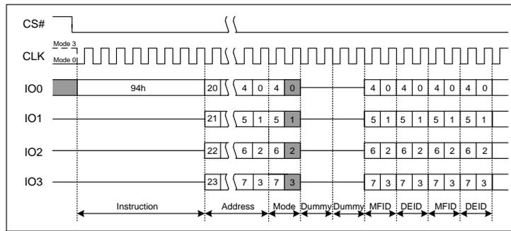
Figure 7.40 Read Manufacturer/Device ID Quad I/O Instruction
