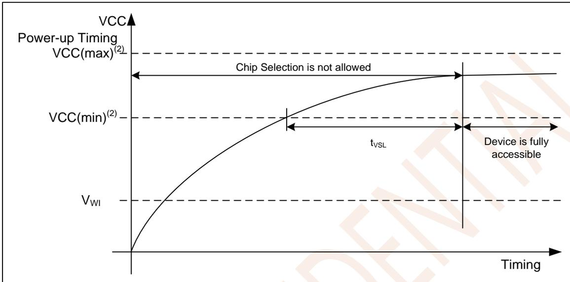
Figure 8.1 Power-up Timing
