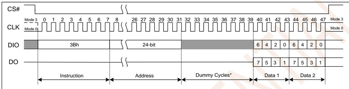
Figure 7.16 Fast Read Dual Output Instruction Sequence Diagram
