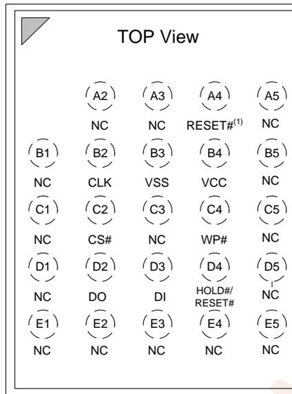
**Figure 3.4 24-BALL TFBGA (5x5 ball array)**
