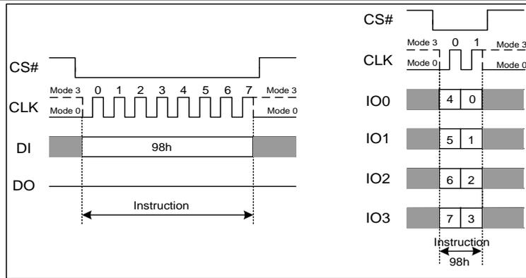
Figure 7.38 Global Block Lock Instruction(SPI or QPI Mode)
