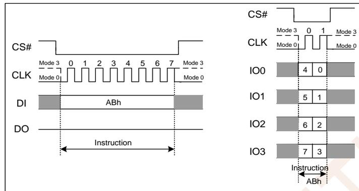
Figure 7.26 Release Power-down Instruction(SPI and QPI Mode)
