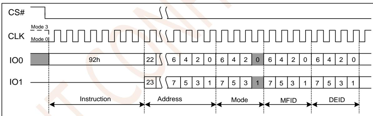
Figure 7.39 Read Manufacturer/Device ID Dual I/O Instruction
