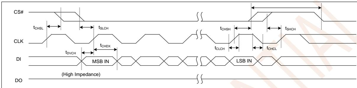
Figure 8.5 Input Timing
