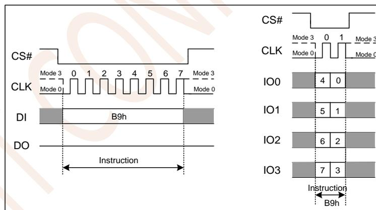
Figure 7.26 Deep Power-down Instruction (SPI and QPI Mode)
