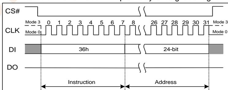
Figure 7.36 Read Manufacturer/Device ID Dual I/O Instruction
