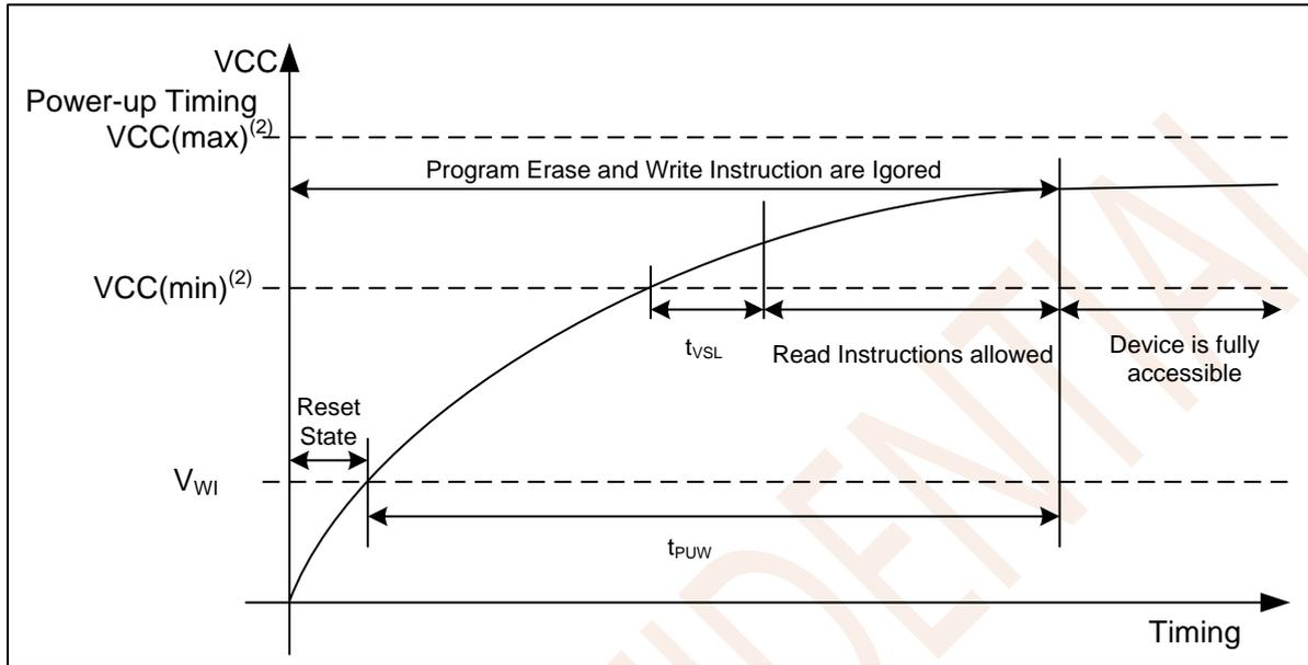
Figure 8.1 Power-up Timing
