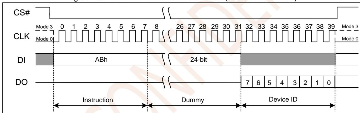
Figure 7.28a Release Power-down / Device ID(SPI Mode)
