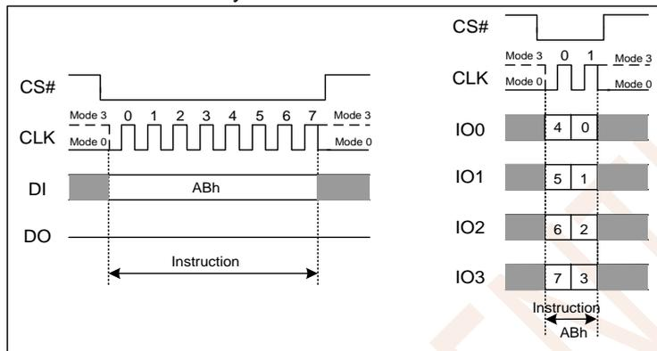
Figure 7.27 Release Power-down Instruction(SPI and QPI Mode)
