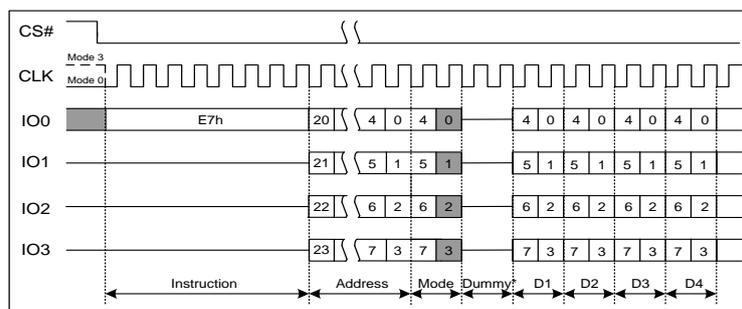
Figure 7.20 Word Read Quad I/O Instruction(Initial command or previous M5-4 ≠10)
