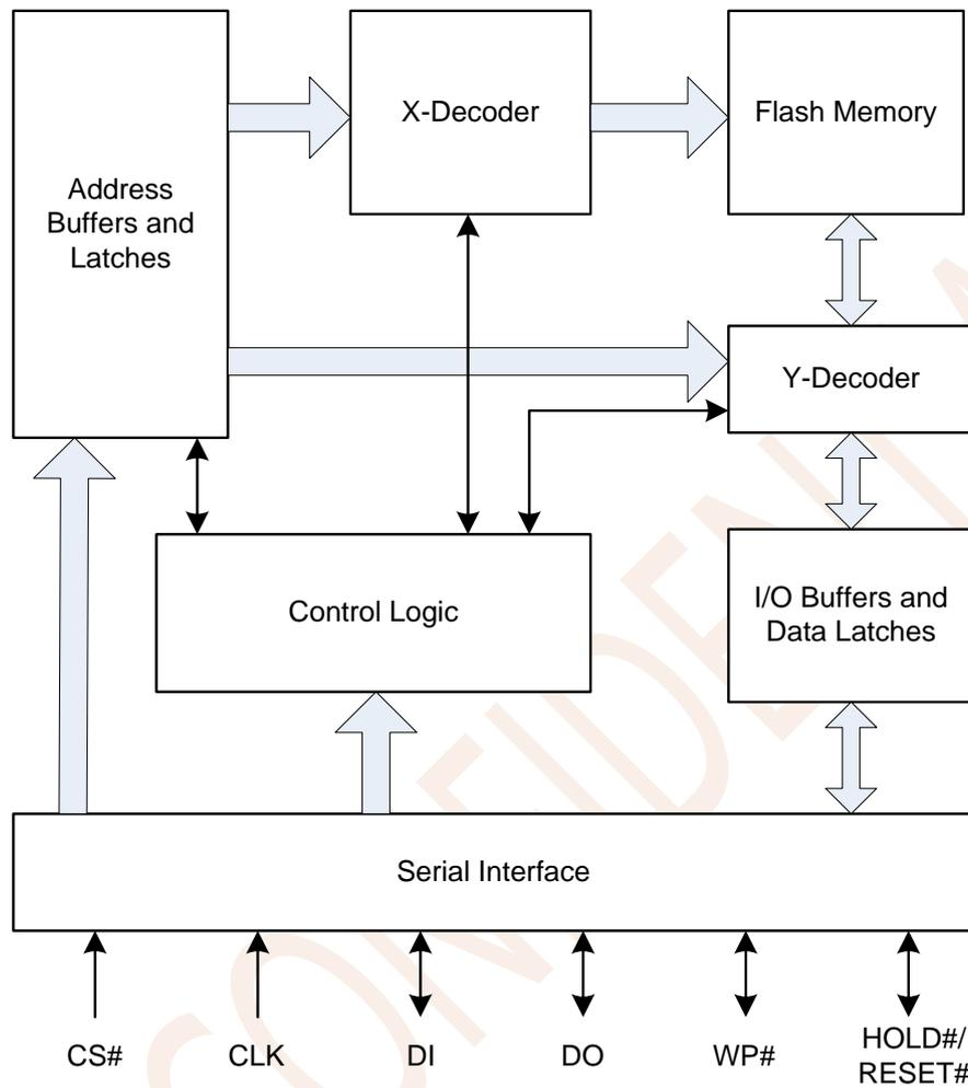
Figure 2.1 Block Diagram
