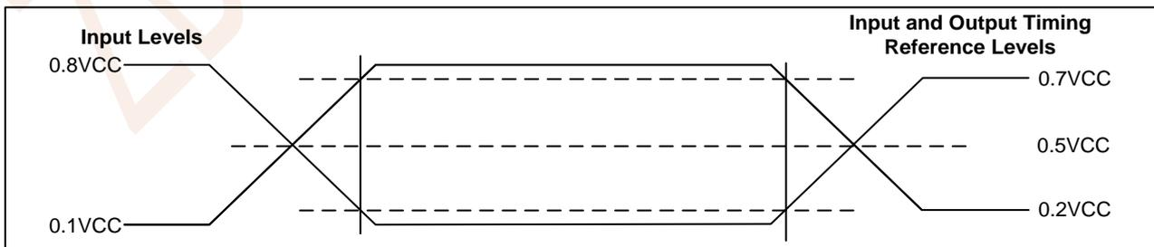
Figure 8.3 AC Measurement I/O Waveform
