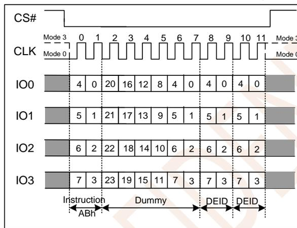
Figure 7.27b Release Power-down / Device ID(QPI Mode)
