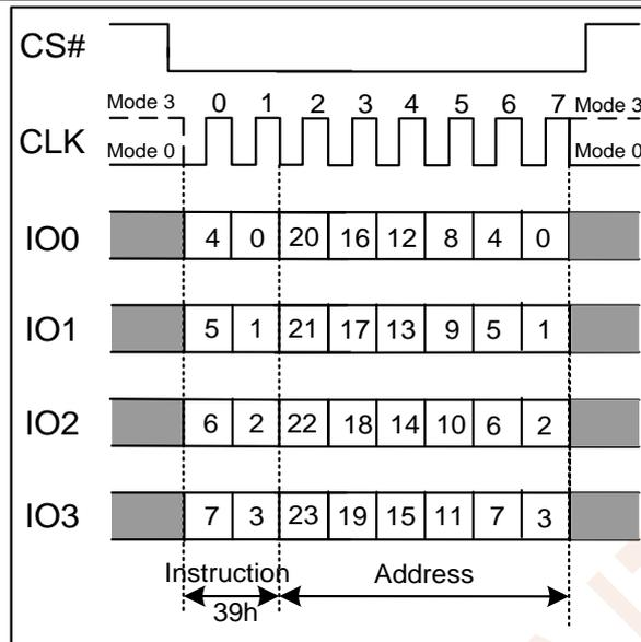
Figure 7.41b Individual Block/Sector Unlock Instruction(QPI Mode)
