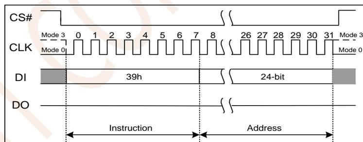
Figure 7.41 Individual Block/Sector Unlock Instruction(SPI Mode)
