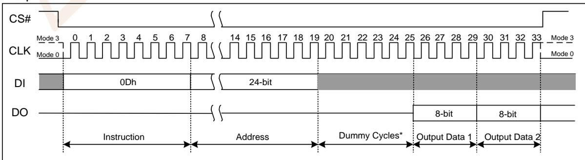
Figure 7.15a DTR Fast Read Instruction (SPI Mode)
