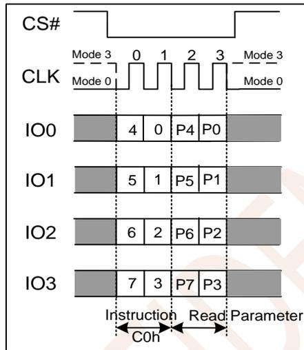
Figure 7.37 Set Read Parameters Instruction (QPI Mode only)
