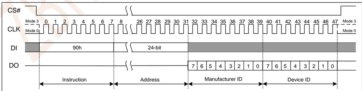
Figure 7.28a Read Manufacturer/Device ID(SPI Mode)
