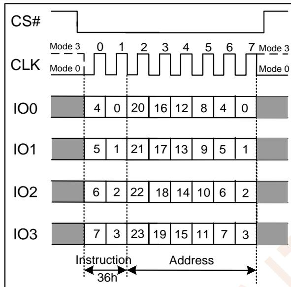
Figure 7.40b Individual Block/Sector Lock Instruction(QPI Mode)
