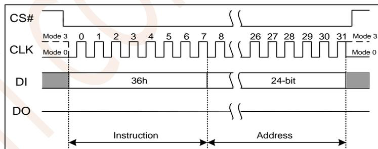
Figure 7.40a Individual Block/Sector Lock Instruction(SPI Mode)
