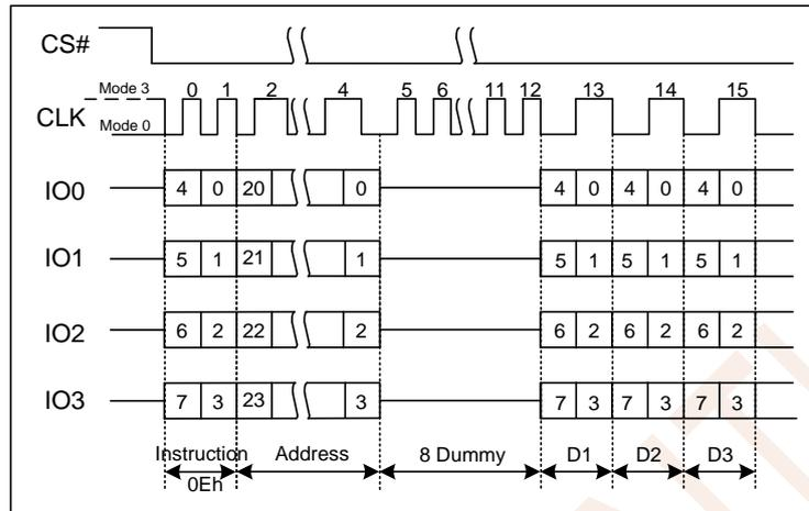
Figure 7.39 DTR Burst Read with Wrap Instruction (QPI Mode only)
