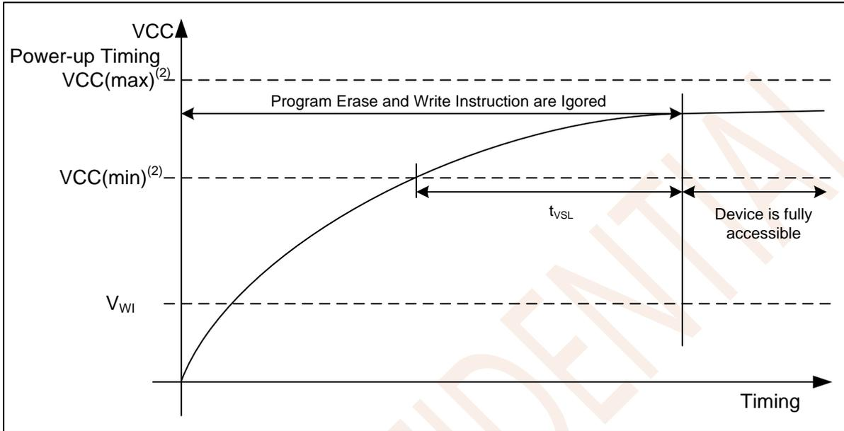
Figure 8.1 Power-up Timing
