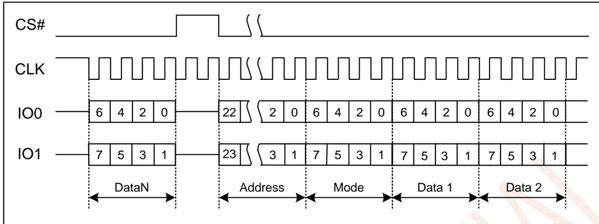
Figure 7.18b Fast Read Dual I/O Instruction (Initial command or previous M5-4=10)
