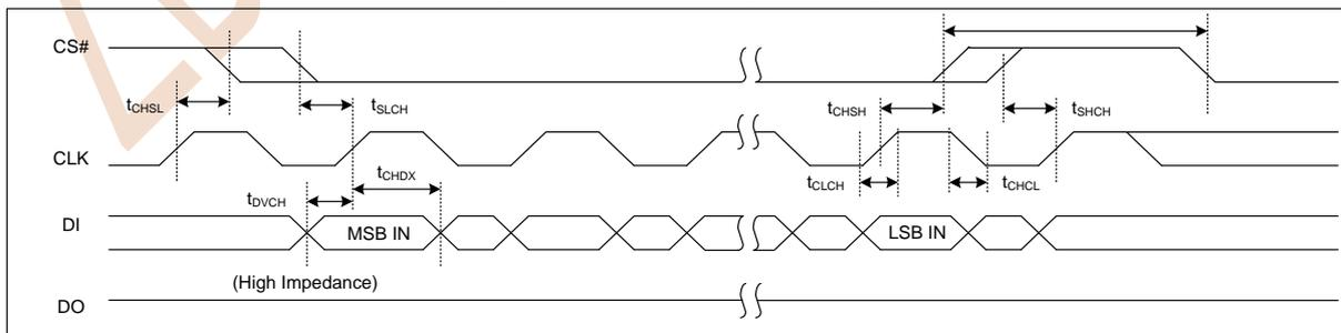
Figure 8.5 Input Timing
