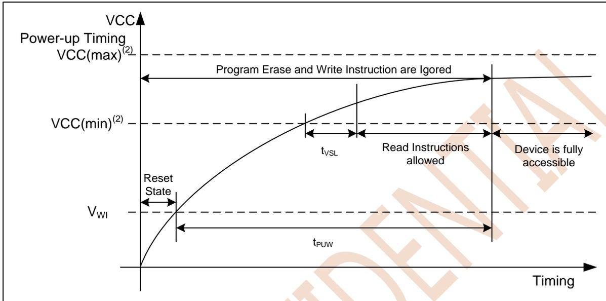
Figure 8.1 Power-up Timing
