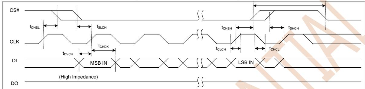
Figure 8.5 Input Timing
